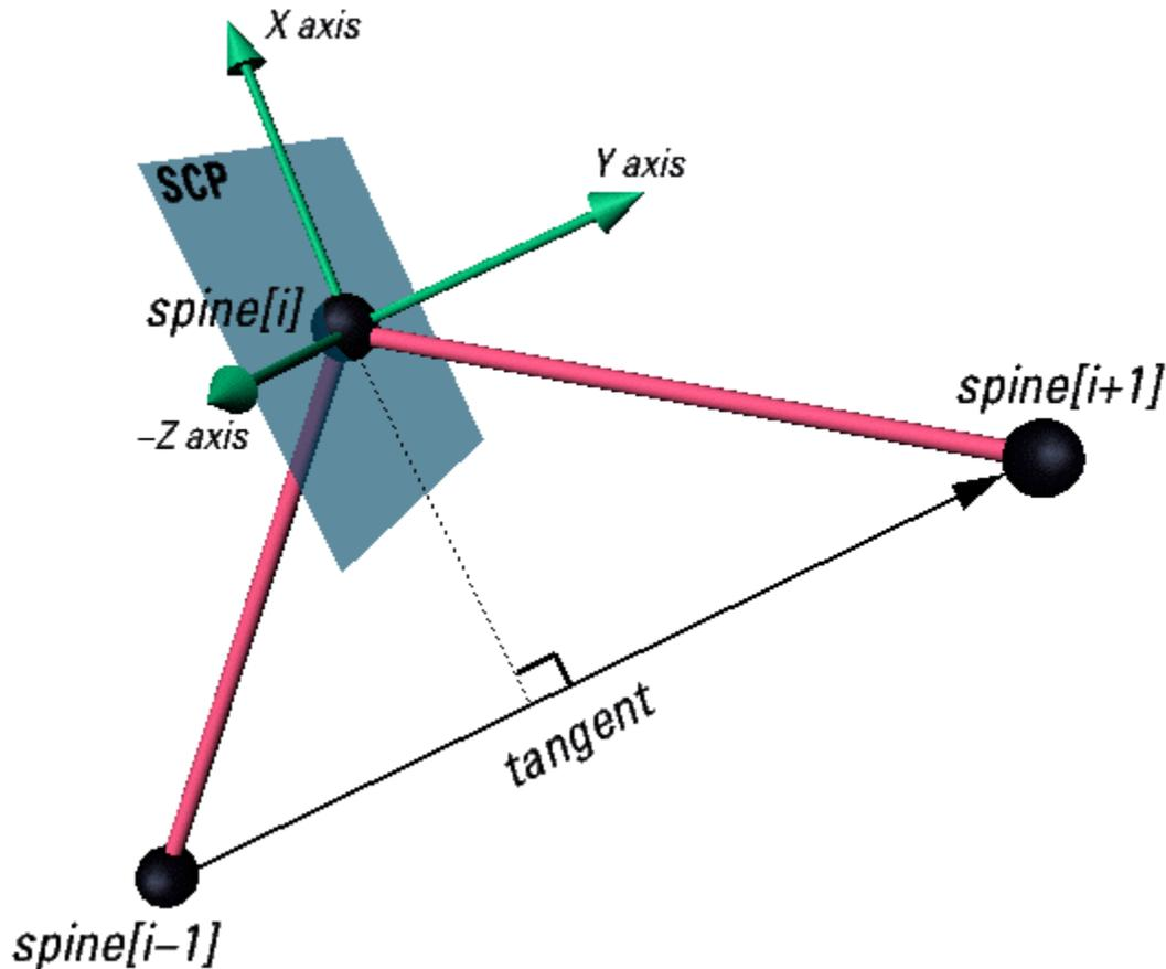
Figure 6.6 -- Spine-aligned cross-section plane at a spine point.
